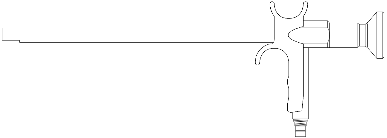
picture 19: Laryngoscope Ø 10 mm, 90°, l=190 mm
